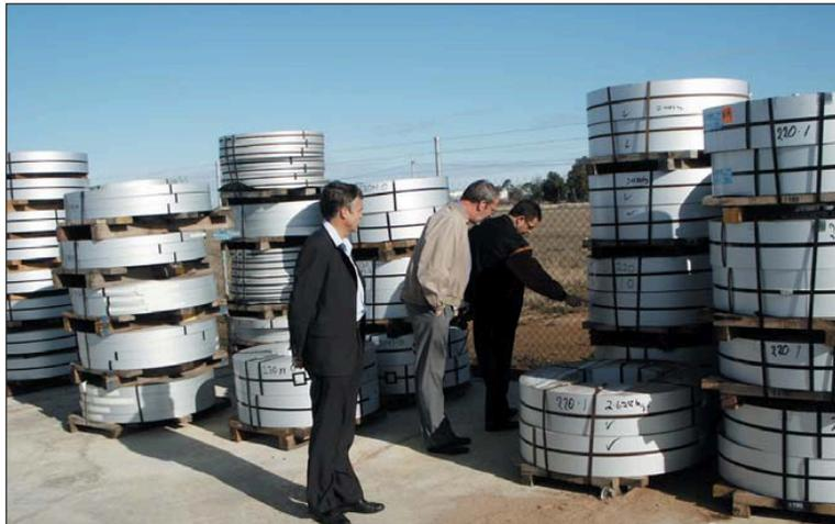
Inspecting stock steel coil strips to be used for subsequent profiling of light weight steel frames in Australia.
